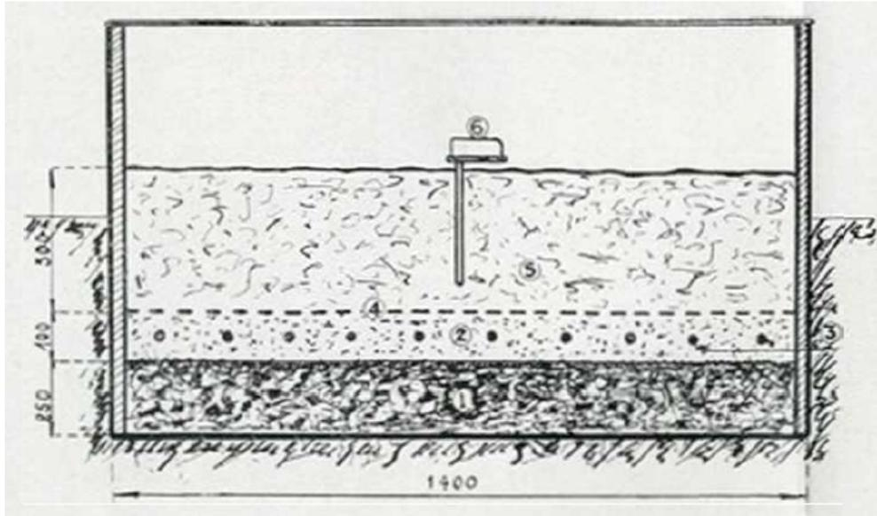
1: slag, 2: sand, 3: heated cable, 4: meshing, 5: potting soil 6: temperature limiter (1936 BIP # 93, Ultimheat Museum)
