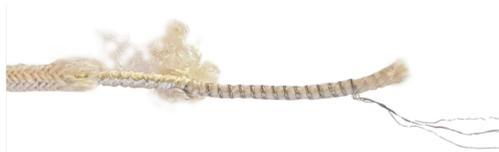
1962 ca, Jidé brand heating cord. Sewn directly onto one of the sides of the heating blanket, no longer between two fabrics, it has four spiral nickel conductors on a cotton core, which are then covered with a very fine wrapping, and then with a cotton braid. The unit is not waterproof and very combustible.
