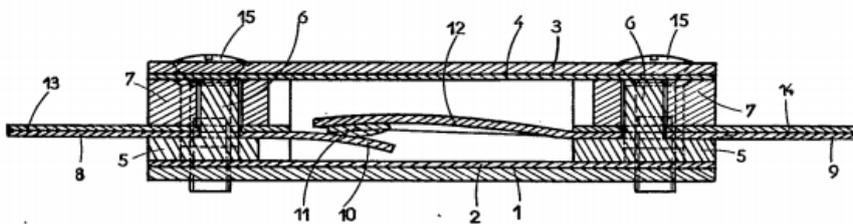
1961 bimetallic miniature snap switch for heat blankets, joint patent of Sté Auge et Cie and Imphy sa No. FR1296066 (France)
