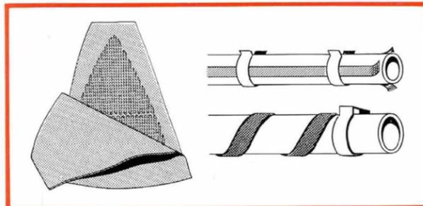
Fabrics and flexible heating fabrics made of glass cloth (1966 Electric Heating Resistors, Ultimheat Museum)
