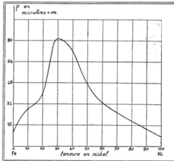
Variation in resistivity: curve versus nickel content in ferro-nickel alloys (La Nature, 1934, Nickel alloys and their applications, P215)
