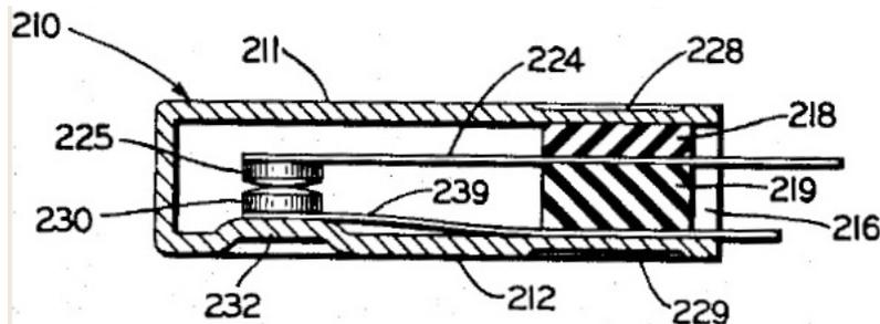
Portage Electric Slow-Breaking Thermostat Models, 1963 (Glenn Wehl US Patent No. 3,223,808)
