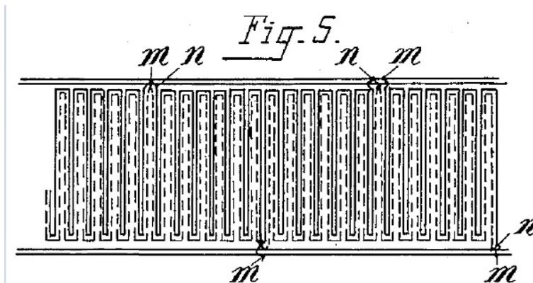
m, n: Detail of the connections on the supply wires in the selvages. This technique is still used today in electrical tracing (patented by Camille Hergott in 1901).
