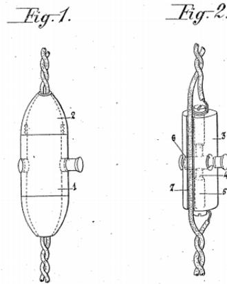
1924 Switch for flexible wires (Patent Arzens75051). In 1933 Calor develops a similar model with snap-off technology
