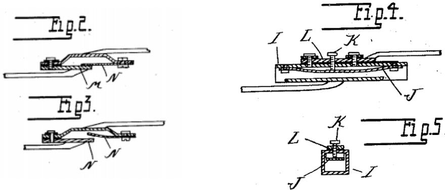
1912 Hoffmann fusible alloy limiter for heating blanket (US Patent 1096916). The fusible alloy welds together blades M and N
