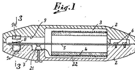
In 1954, Maurice Pierre Marchal working at Tisselec, filed a patent for a bimetallic switch. This product used a small series resistor (No. 22) on the heating blanket and slowly heated a bimetallic strip (5). The aim of this invention was to create a heat timer that automatically turns off heat after a certain duration. Marchal completely failed to achieve gradual heating control, although his system came very close to this idea.
