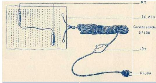
1947 Thermoplasma Calor, view of the heating part with its two protected sheath thermostats (RT) and its 3-position switch (IRT). (Cat Ultimheat)
