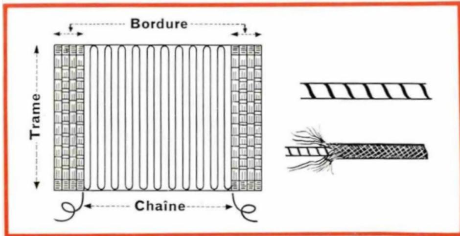
Asbestos heating fabric, and asbestos heating cord and braid (Electric heating resistors, 1966, Ultimheat Museum)
