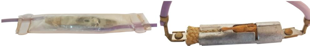
Slow-breaking heating blanket temperature limiter, used in conjunction with an English power control system made by GEC (General Electric Company). It is covered with a waterproof PVC sleeve, welded to the wires. Around 1970 (Ultimheat Collection)
