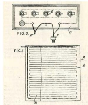
Inside view of the heating mat, top left - wires crossed by the current, bottom right – power socket (1904, La Nature, Ultimheat collection) In England in 1906, RF Lafoon put forward the concept of adjusting the power by placing parallel warning lamps on the resistors (Patent dated October 13)
