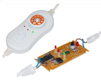
2019 Continuous Electronic Power Control Blanket Control Unit (Ultimheat Collection)
