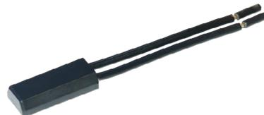
2019 Snap-off temperature limiter for heating transformer, derived from the 1966 Texas Instruments 7AM model, usable at 230V, in plastic waterproof casing. Temperature range of 5 to 8°C. Type V7AM. (Ultimheat Collection)
