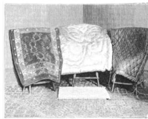
‘Thermoplasme Parvillée’ 1903. Dimensions 25cm x 35 cm Power: “Less than that of 5 candle lamps” or about 50 watts (at this time). The surface charge was around 0.06 W / cm 2. By 1904, Camille Hergott had commercially released heating carpets and electric blankets using the technology of his inventions (1904, La Nature, Ultimheat Collection)
