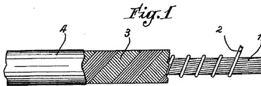
As early as 1949, Tissélec filed a first patent for a heating cord whose outer covering (3) was covered with a rubber, pvc or polyethylene type elastomer (4) in order to improve insulation, particularly in cases where the cover was wet. (Patent FR 982675 registered on June 13, 1951)
