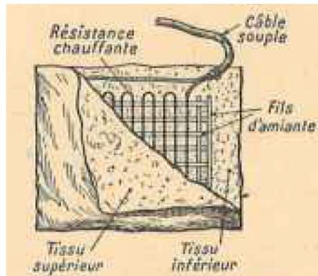
The following passage on personal heating is from 1932: Heated fabrics in the form of carpets, slippers, blankets, knitwear, jackets, ... where the heating resistance (50 watts) is insulated by two asbestos wires, woven between two layers of fabric (1932 Boll, Electricity to the City and Countryside)
