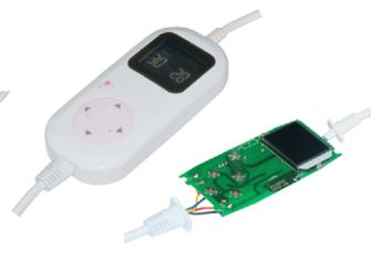
2019 Control unit for temperature-controlled heating blankets with digital display via a thermistor probe incorporated into the heated area (Ultimheat Collection)
