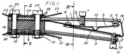
1944 Thermega fast break limiter for heating blankets
