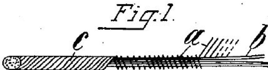
Heating cord (patented by Camille Herrgott, 1901). A = heating wire; B = textile core; C = outside wrapping wound in the opposite direction of the heating wire
