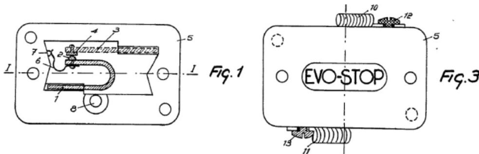
In 1957, Maurice Georges Moïse Gervaiseau, a thermoplastics manufacturer (151 Georges Durand Avenue, Le Mans), developed a compact bimetallic thermostat, under the brand name Evo-Stop, in a closed unit with an improved slow breaker, in order to overcome the problem of radio interference and was specifically intended for heating blankets. (Patent 1169253)
