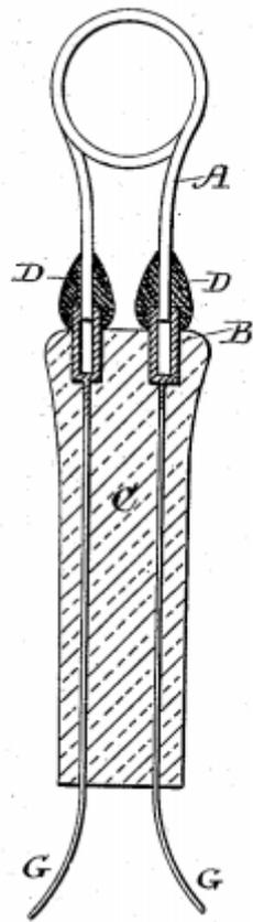
1881 carbon filament lamp, improved methods of connecting the filament to the electrodes ( English Patent No. 4.202 of 29 September 1881, by Joseph Wilson Swan)
